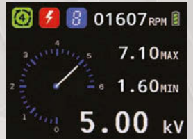
Analog gauge and digital readout with maximum and minimum
