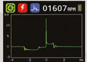
Displays secondary ignition waveforms
