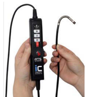
▲ Accessing the back of the intake valve to observe how much carbon is built up on the valve stem and back of the valve usually involves removing the intake plenum then inserting a borescope, like the ATS IC Inspection Camera, into the intake valve area.
