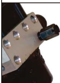
Great for re-threading ABS control modules
