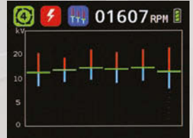
Candle stick graph compares maximum, minimum and average measurements of several cylinders
