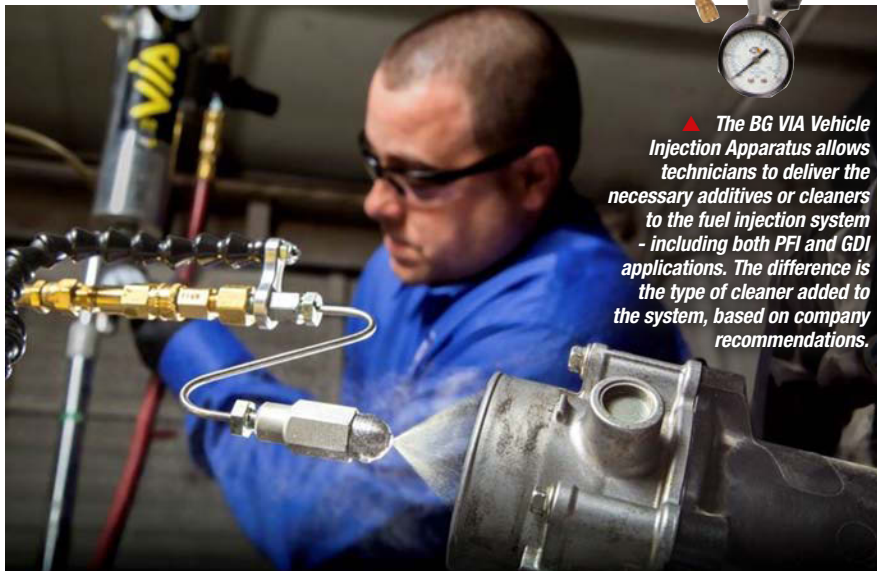
▲ The BG Air Intake System Cleaning Tool, No. 9209, an attachment used on the BG VIA apparatus, finely atomizes BG GDI Intake Valve Cleaner for safe, effective cleanup.
