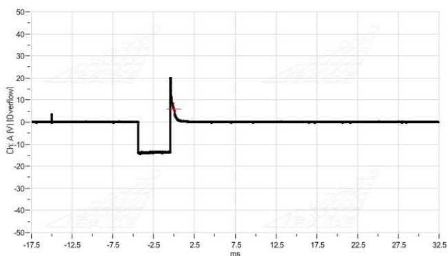
▲ Fig. 3. The waveform showed normal and also indicated the added injector "on time" as indicated by the fuel trim numbers. Note the voltage spike at shut-off. Here, 20V indicates no resistance in the circuit.
