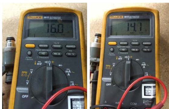
◀ Fig. 5. One injector showed 14.1 ohms (right), while the other has 16.0 (left) ohms resistance. Even though this is a small amount of difference, it can affect the injector's performance, but generally does not indicate a misfire.
