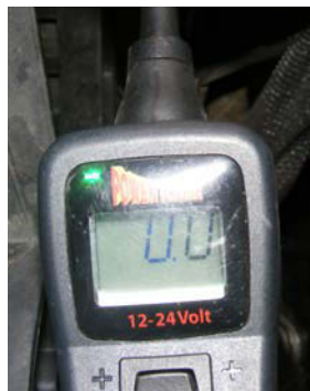
▲ Fig. 2. Using the Power Probe III, we found there was no power at the connector, when the scan tool commanded it.
