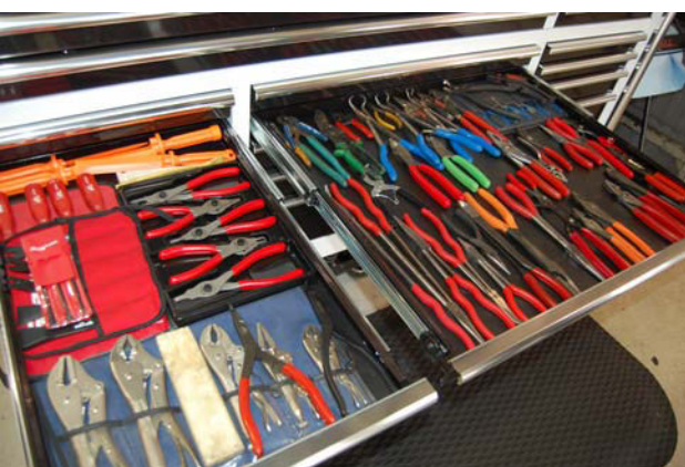
▲ Each drawer of Russell’s box has a slip-proof mat that holds tools in place, which helps him stay organized.
