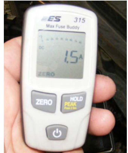
▲ Fig. 4. As a final check, use an ESI 315 Fuse Buddy placed into the A/C fuse to make sure that the amperage to the compressor is within specifications. For information on this product, visit: VehicleServicePros.com/10103238
