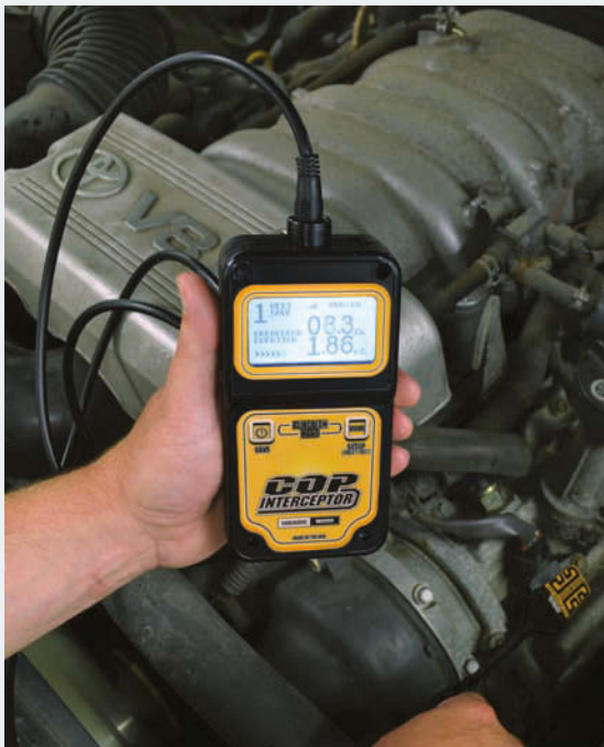
▲ The COP Interceptor measures, displays and can save each coil on plug’s secondary ignition data in real-time for detailed ignition analysis.
