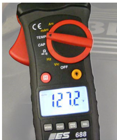
▲ Fig. 5. Use a temperature probe, like the Electronic Specialties 688, and your DMM, on the evaporator inlet (left) and outlet (right) to make sure that there is no more than a +/-5 degree F difference in temperature.
