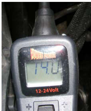
▲ Fig. 3. We disconnected the connector and checked for power again. We found that with it disconnected, voltage showed when the PCM commanded it, but we lost it when we connected to the clutch.
