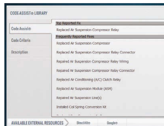
▲ The Genisys Touch from Bosch OTC displays the appropriate vehicle information when the user has read the code and taps on the DTC to show the AutoDetect results. For information on this tool, go to: VehicleServicePros.com/10820435
