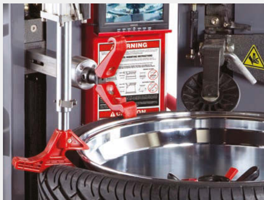
The Ranger RX3040 can pull the bead over the wheel without ever touching the rim. For more information on this product go to VehicleServicePros.com/10106963 .
