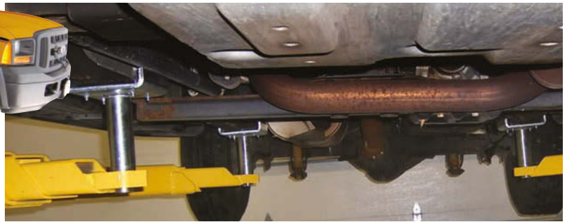
Frame-cradling adapters are recommended for two-post lifts.
