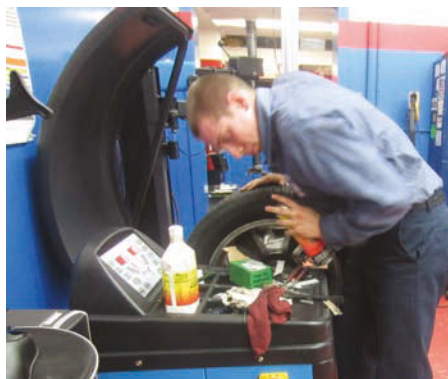
The old school way of balancing a tire: here, a tech lines up the tire with the naked eye and cleans off a spot to put on "sticky weights."
