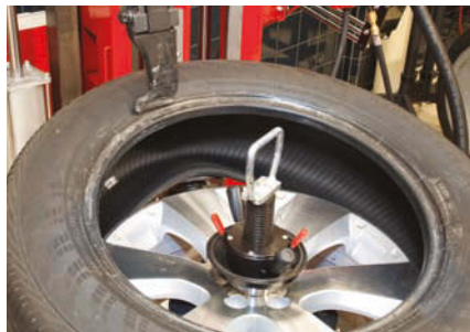
The Hunter Auto34 removes the bottom bead of the tire from the rim without the use of a tire bar. For more information on this product, go to VehicleServicePros.com/10101463 .
