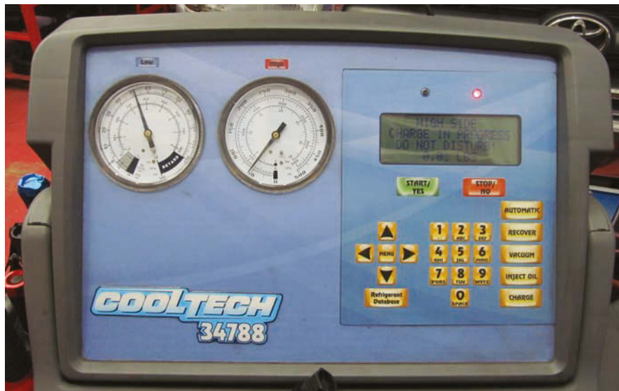
▼ Fig. 2: After a leak test, the vehicle will quickly suck up refrigerant from the machine. After doing this, many machines, like the Robinair Cooltech 34788, will inject oil into the vehicle. An oil with dye already in it will assist in diagnosing any possible future A/C leaks.
