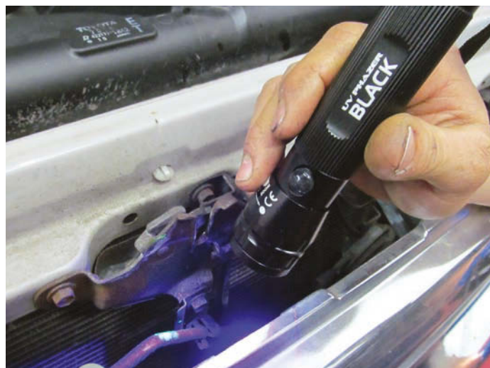
▼ Fig. 7: Dye was found on this high side A/C line with a UView Phazer Black. For more information on this tool go to VehicleServicePros.com/10843246 .
