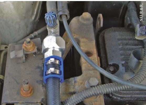
▲ An example of a real-world A/C hose repair with the S.U.R.&R. AC1387 Deluxe A/C Line Repair Kit. For more information on this product check out VehicleServicePros.com/10237246 .
