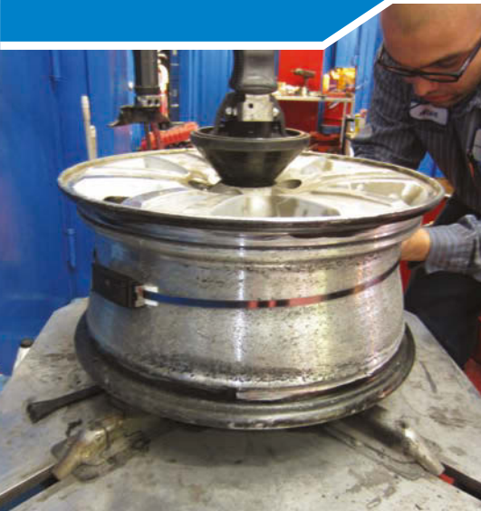
The ingredients to a no-comeback tire job on a Ford Explorer with aluminum rims: sanding the rim down, painting on bead sealer, lubing the new valve stem and the tire itself with non-corrosive tire lubricant and, on this vehicle, properly replacing the broken TPMS sensor.
