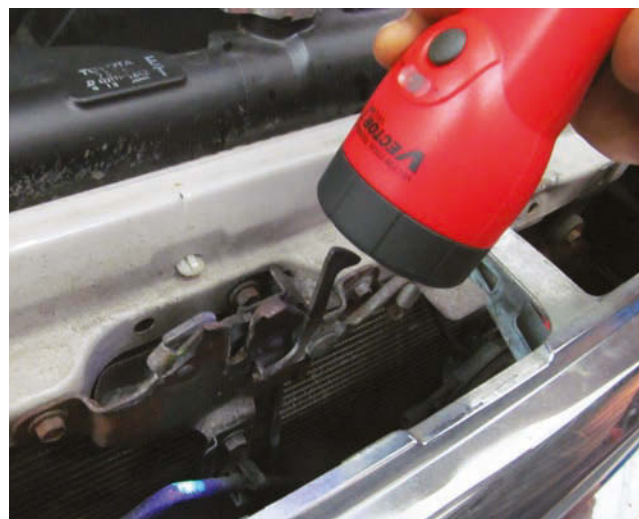
▼ Fig. 8: Here, the Cliplight Vector 7 shines light on the same A/C leak. An interesting feature of this tool is that it does not shine brightly, yet the dye does. For more information on this tool go to VehicleServicePros.com/10125895 .
