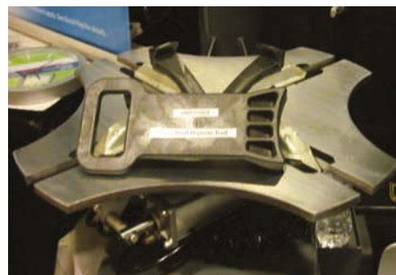
A bead depress tool from Bosch, No. SM103264 assists in pulling the tire over the rim.
