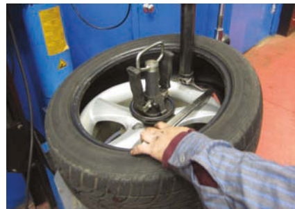
Using a standard tire machine, a tire bar must be wedged between the top front part of the mount/demount head and the tire itself when removing the tire from the rim.
