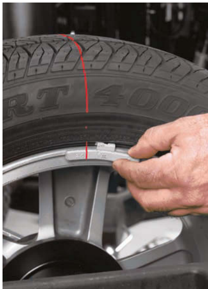
New high-end tire balancers use a laser to guide you where to position the weight, even moving the tire into position for weight placement.
