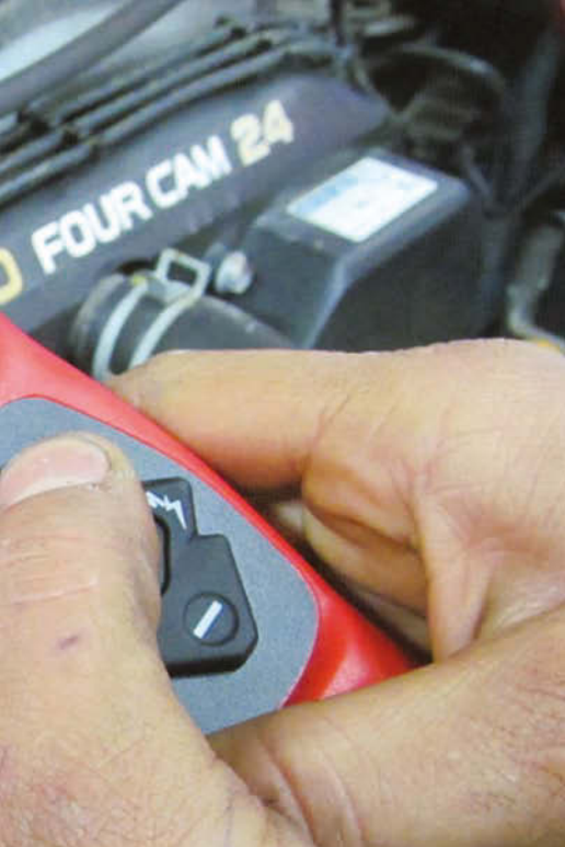
▲ Fig. 4: The PowerProbe Hook, here jumped to the power side of the A/C compressor, can quickly turn the compressor on in order to confirm the it is in working condition. This Toyota 4Runner compressor pulls a about 2.5 amps even though it has a 10-amp fuse. For more information on this tool, go to VehicleServicePros.com/10727921 .
