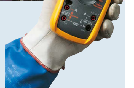
Proper safety equipment should be used with a Fluke 1587 insulation-test capable multimeter.
