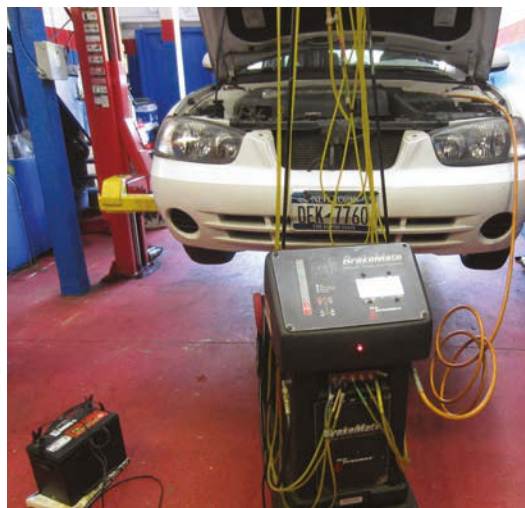
Bleed the brakes with a brake flush machine. Notice that a battery is not directly on the floor. This is in accordance with EPA regulations in order to prevent fines. For more information on the Flo-Dynamics BrakeMate Jr., check out VehicleServicePros.com/10106064 .
