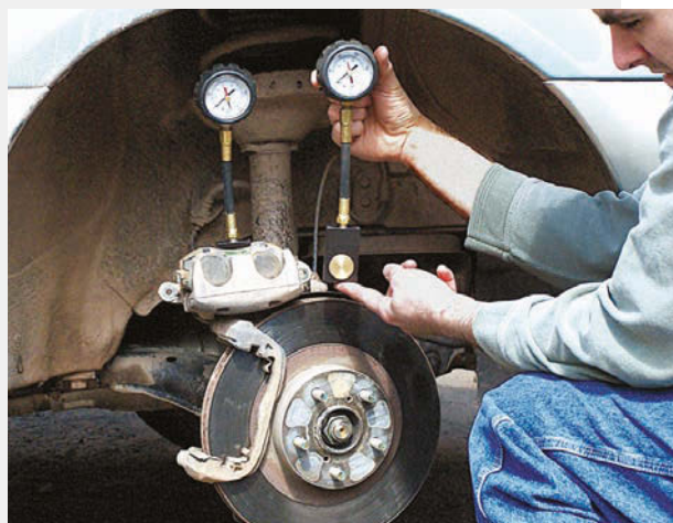
Testing a brake caliper with a Disc Brake System Analyzer from Innovative Products of America requires removing the caliper and putting the gauge in between the brake pads. For more information on this tool, check out VehicleServicePros.com/10877983 .
