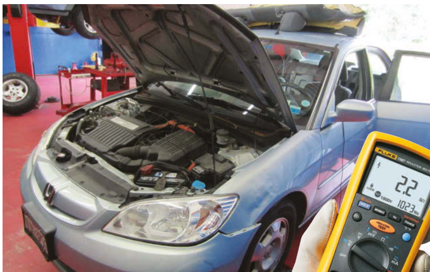
Figure 1: This 2005 Honda Civic Hybrid has an IMA light on. In order to access the HV battery, the rear seat has to be removed.
