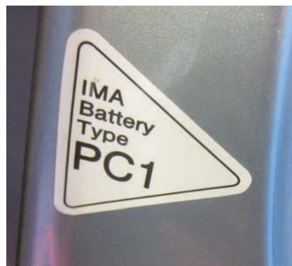
Fig. 5: These stickers saying "PC1" are put on Honda hybrids with an updated HV battery.
