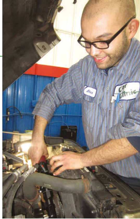
Portillo demonstrates how the cordless ratchet can get into a tight spot.
