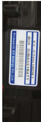
Fig. 1: The new HV battery the dealer installed into this 2006 Honda Civic Hybrid.
