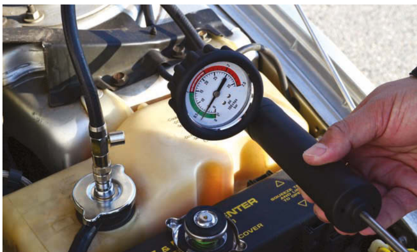
Any pressure tester worth its salt, such as Astro Pneumatic's Radiator Pressure Tester, No. 78585, shown here, will have the right adapters to connect to vehicles that have pressurized caps on their coolant overflow reservoirs. For more information on this product, go to VehicleServicePros.com/10166850 .
