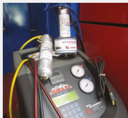
Figure 3: Here is a real-world A/C setup. Pictured is an A/C machine (from Flo-Dynamics) and two "filters" that hook up to the hoses when needed. What these "filters" do is different. Both made by Airsept, one prevents PAG oil contamination in hybrids and the other filters out sealant that can damage your machine. For more information on these products check out VehicleServicePros.com/10106929 (Charge Guard) and VehicleServicePros.com/10307871 (Recycle Guard). To learn more about the A/C machine from Flo-Dynamics, go to VehicleServicePros.com/10097576 .
