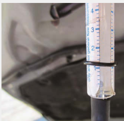
Figure 2: After three minutes, if the ball falls enough, there is malicious sealant in the system. SAE 2670 sealant should not cause a failure when tested with a sealant detection kit. If so, the sealant should be properly removed from the vehicle.
