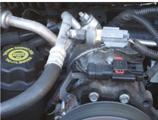
Figure 4: A Jeep Liberty A/C compressor in “normal vision.”
