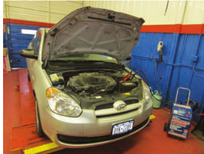
Fig. 2: A battery maintainer, not charger, should be on a vehicle at all times during a reflash. Check out the Associated Equipment Intellamatic battery charger, No. ESS6008MSK, at VehicleServicePros.com/10731899 .
