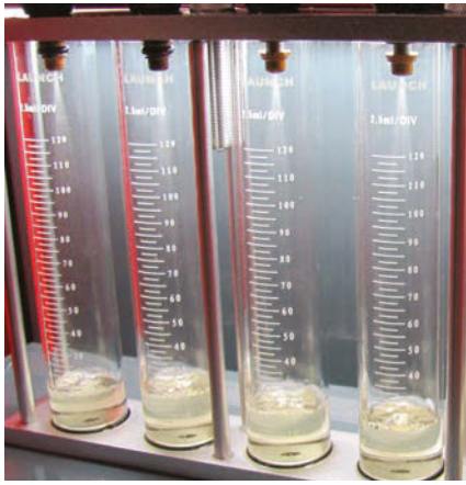
Fuel injectors are flow tested to see if there is a problem. If there is, in most cases the ultrasonic cleaning function of the Launch X-SonicClean is able to break up any hard deposits while running its automated cleaning. For information on this product, go to www.VehicleServicePros.com/10225061 .
