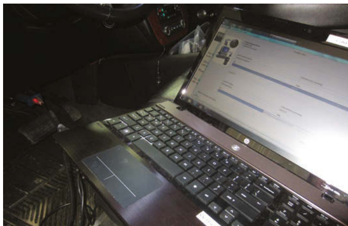
Fig. 3: A GM is reflashed using an AC Delco subscription with a Drew Tech Mongoose cable. Mongoose cables allow the user to use J2534 technology in order to turn their PC into the factory scan tool. Check this tool out at VehicleServicePros.com/10760444 .
