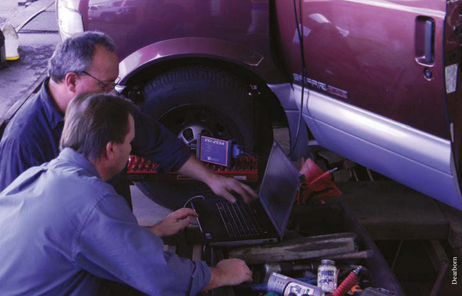
Fig. 4: An example of a properly set up vehicle. Pictured here is DG Technologies' DPA5, an example of a J2534 and RP1210 reflasher, which allows the unit to reprogram even heavy-duty applications. Check this tool out at VehicleServicePros.com/10774670 .
