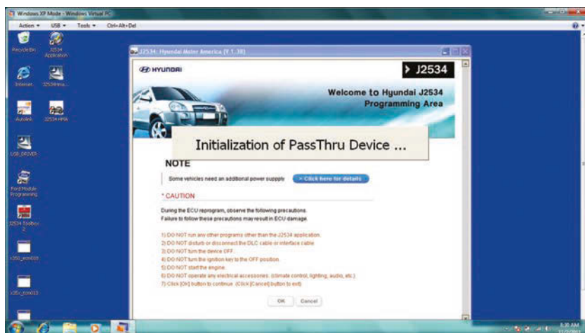
Fig. 5: Note that no other programs are running in the background during this reflash. Also note that Hyundai and KIA factory information and reprogramming software is free and very easy to use.
