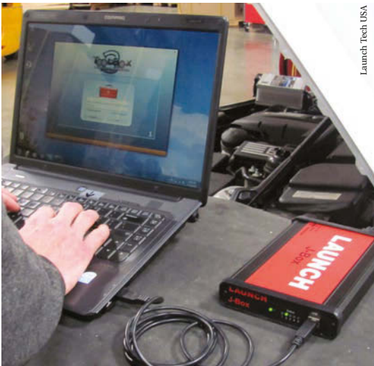
Fig. 1: Drew Technologies makes VIN rewriting software that can be used with its J-2534 hardware. Pictured is Launch's “J-Box” with a proprietary 20-pin connector. The connector allows the J-Box to be used as a factory interface on older Bimmers when purchasing the factory subscription. Check this tool out at VehicleServicePros.com/10782927 .
