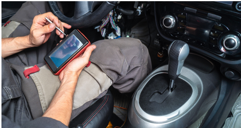
Figure 2 — Preliminary data like a DTC scan can help determine where to begin a diagnosis but should only be used as a piece of the diagnostic puzzle.
