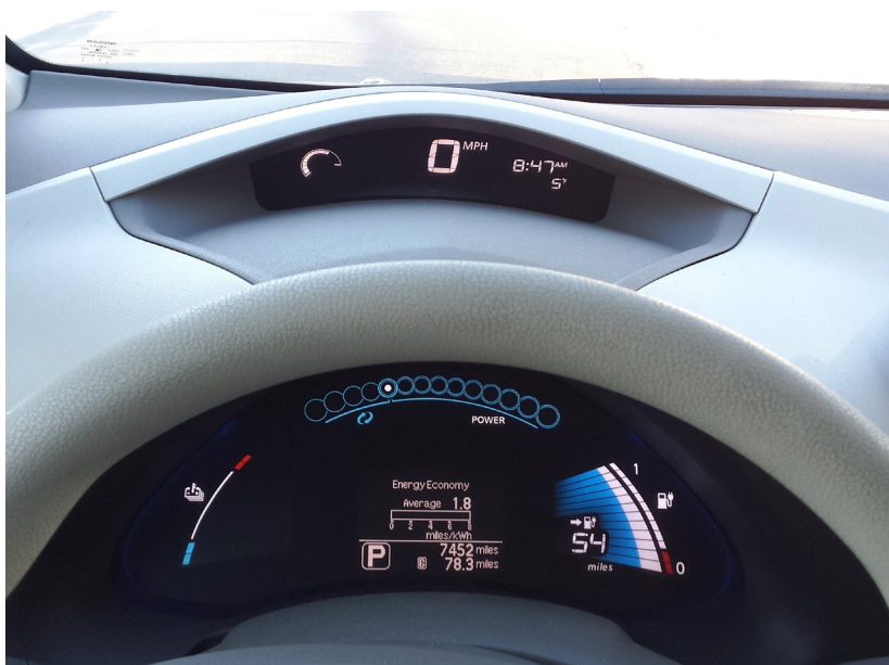
A no-READY light on a Nissan Leaf (simulated). Photo courtesy of ACD
