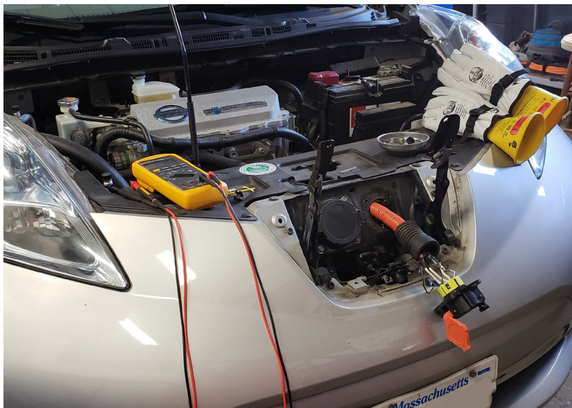
Nissan Leaf that will not charge on a Level II EVSE. Photo courtesy of ACDC
