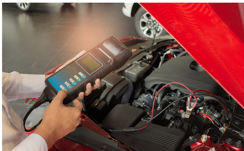
Figure 1 — A capacitance tester is commonly used to quickly evaluate the condition of a battery. However, I have witnessed many “pass” a failed battery. Capacitance is simply one characteristic of a battery’s performance.
