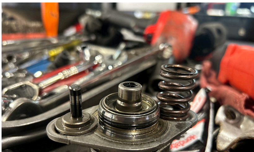
Figure 7 — On the left of the HPFP you can see the HPFP rod, and on the right, you can see the spring. In the middle, you can see the hole where seven gallons of fuel drained out of the high-pressure system.
