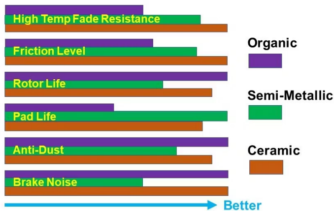
Figure 7- This chart shows relative performance comparisons between organic, semi-metallic and ceramic brake pads. Specific aftermarket and OE pad characteristics may be different than illustrated.
