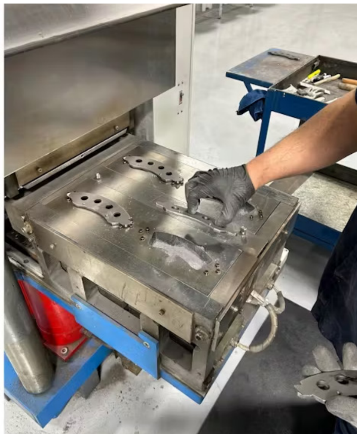
Figure 9- This machine is a positive mold tool and friction hot press. The pad material mix is poured into the mold cavity and cured using heat and pressure. A set of brake pads can be pressed and cured (heated) in about five minutes.
