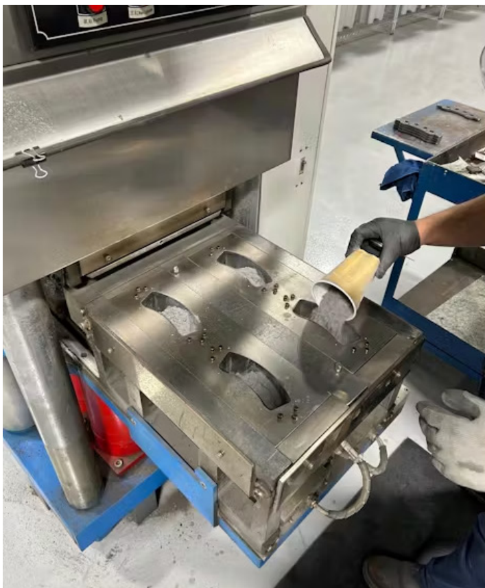
Figure 9- This machine is a positive mold tool and friction hot press. The pad material mix is poured into the mold cavity and cured using heat and pressure. A set of brake pads can be pressed and cured (heated) in about five minutes.
