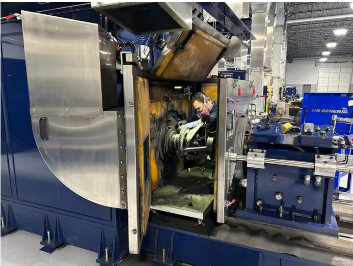
Figure 5- A technician tests brake pads with this Link Engineering brake dynamometer that simulates driving conditions and assess stopping ability, noise, durability and heat ranges of brake pads.
