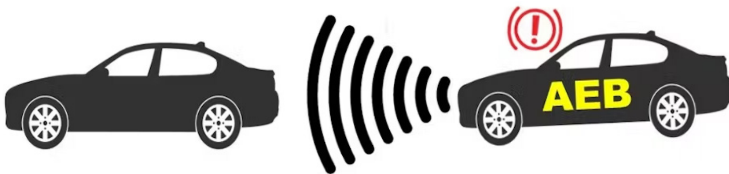
Figure 2- A vehicle's automatic emergency braking (AEB) system is triggered when its radar indicates an imminent collision. Are the brake pads your shop installs up to this task?
