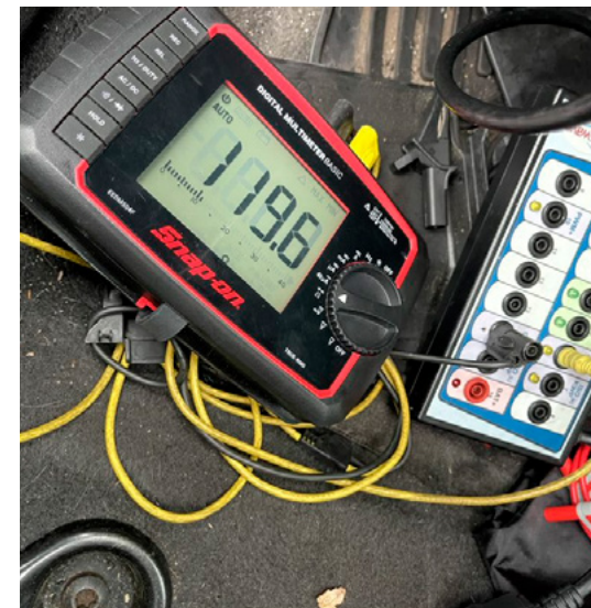
▲ Figure 3 — Resistance test being performed (using my AESWave LineSpi breakout box and Snap-on DMM at the DLC) of the CAN bus.
