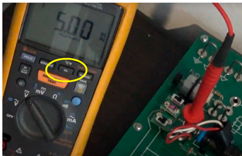
▲ Figure 3 — The meter is displaying a 5 Hz signal, indicating that the injector is being driven five times in one second of elapsed time. Photo courtesy of Brandon Steckler
