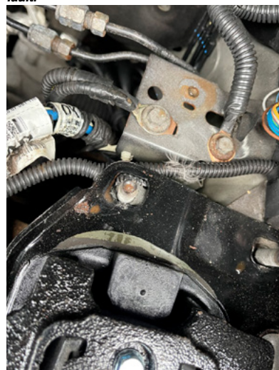
▲ Figure 7 — The harness was caught between the mount and bracket.
