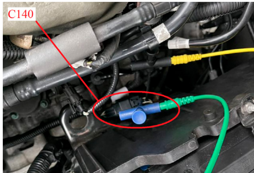
▲ Figure 6 — Connector C140 is a perfect spot to divide the circuit to isolate the location of the fault.
