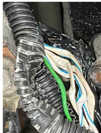
▲ Figure 8 — The damage to the harness, visible after it was freed from the bracket.
